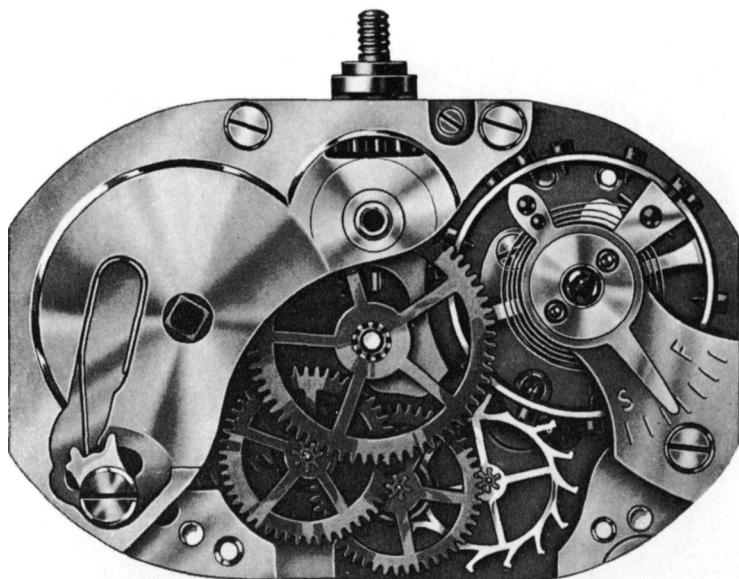
Plate III: Train wheel bridge removed.
